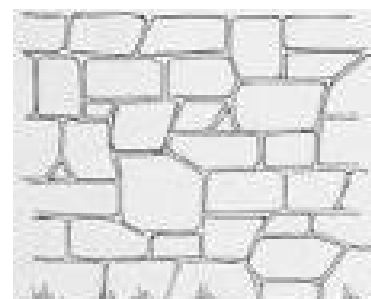
Fig.1.9: Uncoursed Rubble Masonry
